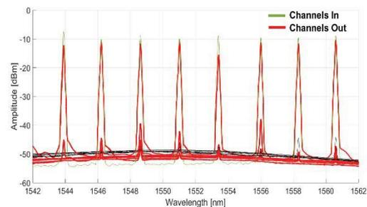
Fig. 3: Optical spectra of the WDM channels switched by the WSS.
