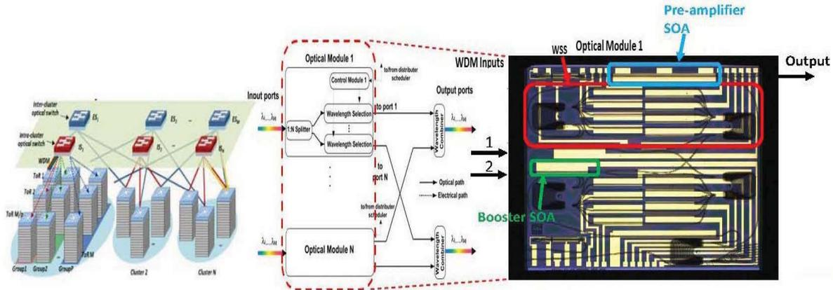
Fig. 1: Schematic of the optical cross-connect.  $N = 2$  optical modules,  $M = 8$  channel wavelengths for the proposed device.
