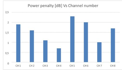
**Fig. 5:** Power penalty for an error-free signal (BER =  $10e-09$ ) at 20Gb/s bitrate.
