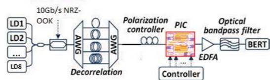
Fig. 2: Experimental set-up employed to assess the performance of the WDM photonic cross-connect.
