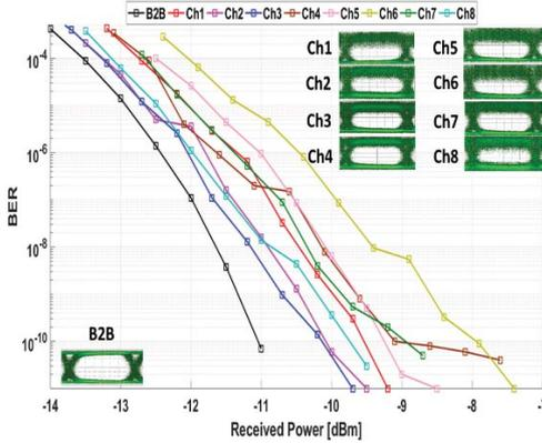
**Fig. 4:** Eye diagrams and BER curves of the switched WDM signals to the output ports of the photonic chip.
