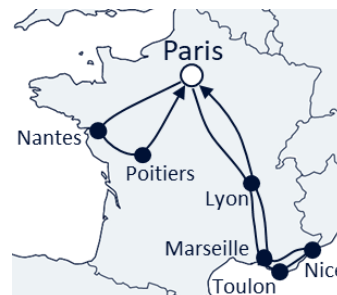
Fig. 1: Field trial performed from Paris network node to 15 PoPs on Orange International Networks Infrastructures and Services (OINIS) network based on Nokia PSE-Vs technology
